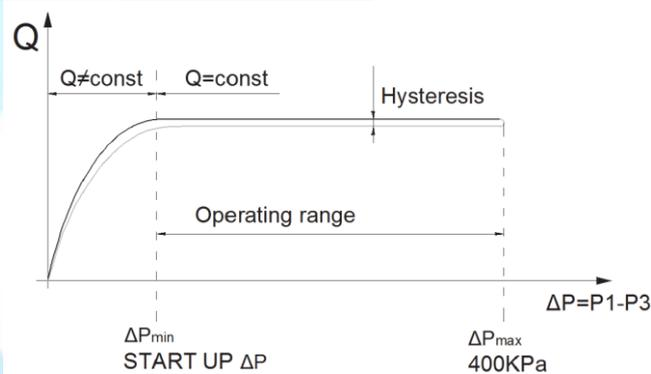
Flow Rate versus Differential Pressure
