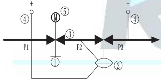
The mechanical series-connected differential pressure controller keeps the differential pressure ( $p_1 - p_2$ ) constant across the control valve and thus the set volumetric flow too. The desired maximum volumetric flow can be preset with the adjusting mechanism. The volumetric flow through the control valve opening to control. The controller (not shown) and the actuator regulate the volumetric flow and consequently the desired temperature in buildings, rooms or zones.
