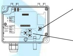
Note: The ZERO button can be operated outside the front cover. It's for resetting zero point. Other buttons and jumpers are on PCB, customers need to open the front cover to operate them.
