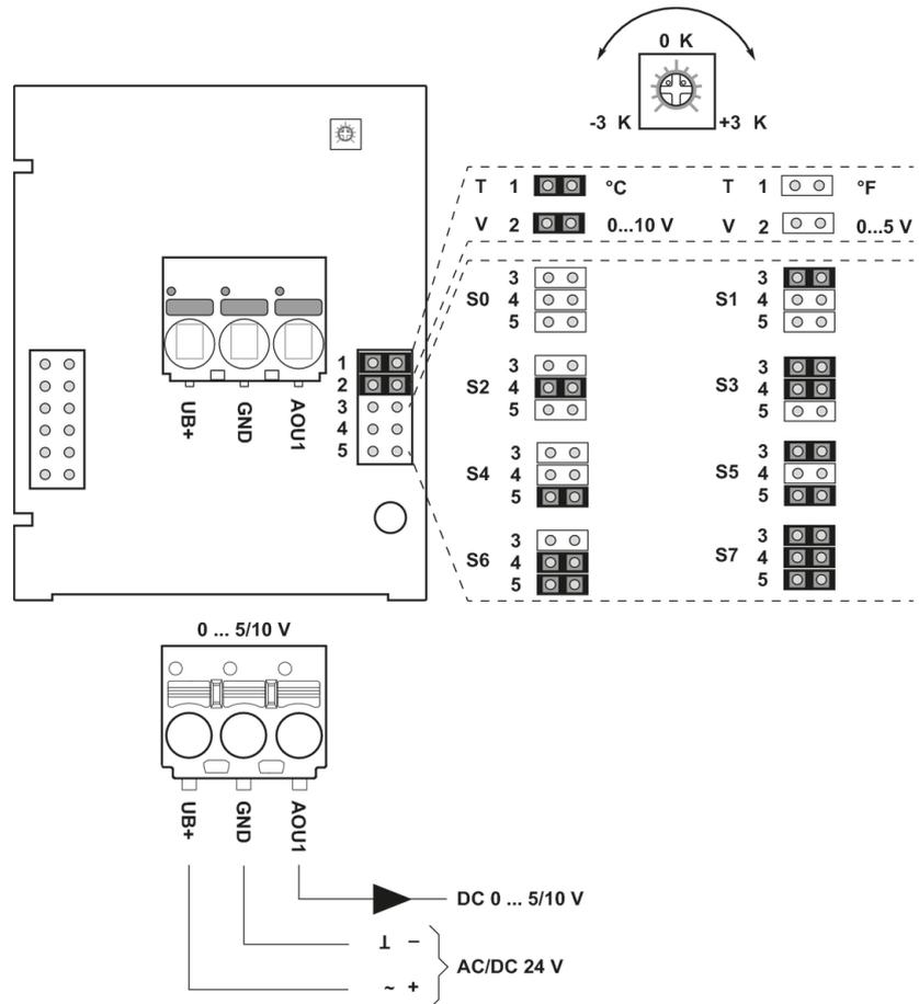
the adjustment of the measuring ranges is made by changing the bonding jumpers
